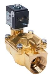
ODE potable water solenoid valve, 2-port (2-way), 2-position, N.C., lead-free brass body, 1in female NPT inlet(s), 1in female NPT outlet(s), Cv=14, 24 VDC operating voltage, 11W, NSF/ANSI 61.
