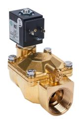
ODE potable water solenoid valve, 2-port (2-way), 2-position, N.C., lead-free brass body, 1in female NPT inlet(s), 1in female NPT outlet(s), Cv=14, 120 VAC (60Hz)/110 VAC (50Hz) operating voltage, 15 VA.
