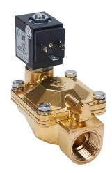
ODE potable water solenoid valve, 2-port (2-way), 2-position, N.C., lead-free brass body, 3/4in female NPT inlet(s), 3/4in female NPT outlet(s), Cv=9.8, 120 VAC (60Hz)/110 VAC (50Hz) operating voltage, 15 VA, NSF/ANSI 61.
