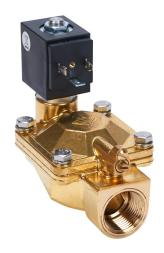
ODE potable water solenoid valve, 2-port (2-way), 2-position, N.C., lead-free brass body, 3/4in female NPT inlet(s), 3/4in female NPT outlet(s), Cv=9.8, 24 VDC operating voltage, 11W, NSF/ANSI 61.
