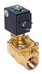
ODE potable water solenoid valve, 2-port (2-way), 2-position, N.C., lead-free brass body, 1/2in female NPT inlet(s), 1/2in female NPT outlet(s), Cv=4.8, 24 VDC operating voltage, 11W, NSF/ANSI 61.
