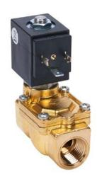
ODE potable water solenoid valve, 2-port (2-way), 2-position, N.C., lead-free brass body, 1/2in female NPT inlet(s), 1/2in female NPT outlet(s), Cv=4.8, 120 VAC (60Hz)/110 VAC (50Hz) operating voltage, 15 VA, NSF/ANSI 61.
