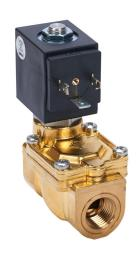
ODE potable water solenoid valve, 2-port (2-way), 2-position, N.C., lead-free brass body, 3/8in female NPT inlet(s), 3/8in female NPT outlet(s), Cv=4.1, 24 VDC operating voltage, 11W, NSF/ANSI 61.
