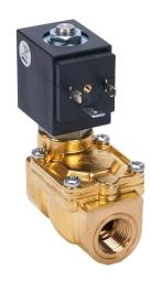
ODE potable water solenoid valve, 2-port (2-way), 2-position, N.C., lead-free brass body, 3/8in female NPT inlet(s), 3/8in female NPT outlet(s), Cv=4.1, 120 VAC (60Hz)/110 VAC (50Hz) operating voltage, 15 VA, NSF/ANSI 61.
