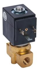
ODE potable water solenoid valve, 2-port (2-way), 2-position, N.C., lead-free brass body, G1/8 female BSPP inlet(s), G1/8 female BSPP outlet(s), Cv=0.63, 24 VDC operating voltage, 11W, NSF/ ANSI 169.
