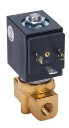
ODE potable water solenoid valve, 2-port (2-way), 2-position, N.C., lead-free brass body, G1/8 female BSPP inlet(s), G1/8 female BSPP outlet(s), Cv=0.63, 120 VAC (60Hz)/110 VAC (50Hz) operating voltage, 15 VA, NSF/ANSI 169.
