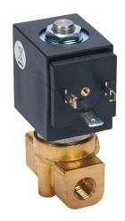
ODE potable water solenoid valve, 2-port (2-way), 2-position, N.C., lead-free brass body, G1/8 female BSPP inlet(s), G1/8 female BSPP outlet(s), Cv=0.63, 120 VAC (60Hz)/110 VAC (50Hz) operating voltage, 15 VA, NSF/ANSI 169.
