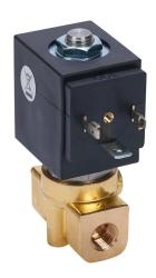
ODE potable water solenoid valve, 2-port (2-way), 2-position, N.C., lead-free brass body, G1/8 female BSPP inlet(s), G1/8 female BSPP outlet(s), Cv=0.22, 24 VDC operating voltage, 11W, NSF/ANSI 169.
