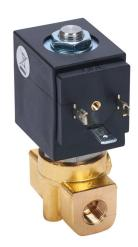
ODE potable water solenoid valve, 2-port (2-way), 2-position, N.C., lead-free brass body, G1/8 female BSPP inlet(s), G1/8 female BSPP outlet(s), Cv=0.22, 120 VAC (60Hz)/110 VAC (50Hz) operating voltage, 15 VA, NSF/ANSI 169.
