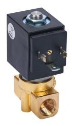
ODE potable water solenoid valve, 2-port (2-way), 2-position, N.C., lead-free brass body, G1/4 female BSPP inlet(s), G1/4 female BSPP outlet(s), Cv=0.63, 24 VDC operating voltage, 11W, NSF/ANSI 169.
