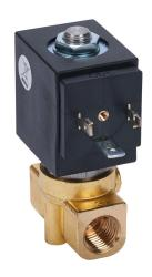
ODE potable water solenoid valve, 2-port (2-way), 2-position, N.C., lead-free brass body, G1/4 female BSPP inlet(s), G1/4 female BSPP outlet(s), Cv=0.63, 120 VAC (60Hz)/110 VAC (50Hz) operating voltage, 15 VA, NSF/ANSI 169.
