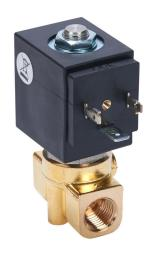
ODE potable water solenoid valve, 2-port (2-way), 2-position, N.C., lead-free brass body, G1/4 female BSPP inlet(s), G1/4 female BSPP outlet(s), Cv=0.22, 24 VDC operating voltage, 11W, NSF/ANSI 169.
