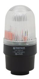
WERMA Xenon tube industrial tall signal beacon, 58mm, clear/white, flashing strobe (0.75 Hz flash frequency), IP65, tube mount, 115 VAC.
