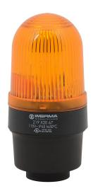
WERMA Xenon tube industrial tall signal beacon, 58mm, yellow, flashing strobe (0.75 Hz flash frequency), IP65, tube mount, 115 VAC.
