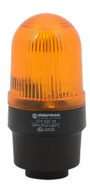
WERMA Xenon tube industrial tall signal beacon, 58mm, yellow, flashing strobe (0.75 Hz flash frequency), IP65, tube mount, 24 VDC.
