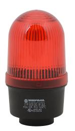
WERMA incandescent industrial tall signal beacon, 57mm, red, permanent, IP65, tube mount, 12-240 VAC/VDC. Requires incandescent bulb.
