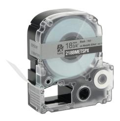
Epson LabelWorks PX series metallic label cartridge, 18mm (3/4in) wide, 30ft roll, black text, silver background, polyethylene terephthalate. For use with Epson LabelWorks PX series label printers.
