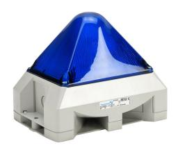
Pfannenberg PYRA series Xenon tube audible-visual signal beacon, 103 dB at 1m, (8) selectable tone(s), selectable flashing strobe, blue, 216 x 144 x 172mm, 24 VDC, IP66, NEMA 4/4X.
