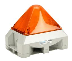
Pfannenberg PYRA series Xenon tube audible-visual signal beacon, 103 dB at 1m, (8) selectable tone(s), selectable flashing strobe, amber, 216 x 144 x 172mm, 24 VDC, IP66, NEMA 4/4X.
