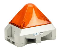
Pfannenberg PYRA series Xenon tube audible-visual signal beacon, 103 dB at 1m, (8) selectable tone(s), selectable flashing strobe, amber, 216 x 144 x 172mm, 24 VDC, IP66, NEMA 4/4X.
