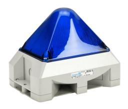
Pfannenberg PYRA series Xenon tube audible-visual signal beacon, 103 dB at 1m, (8) selectable tone(s), selectable flashing strobe, blue, 216 x 144 x 172mm, 115 VAC, IP66, NEMA 4/4X.
