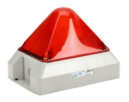
Pfannenberg PYRA series Xenon tube industrial signal beacon, 212 x 144 x 157mm, red, selectable flashing strobe, IP66, NEMA 4/4X, surface mount, 24 VDC.
