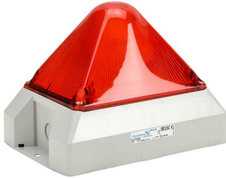
Pfannenberg PYRA series Xenon tube industrial signal beacon, 212 x 144 x 157mm, red, selectable flashing strobe, IP66, NEMA 4/4X, surface mount, 115 VAC.
