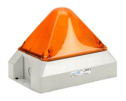
Pfannenberg PYRA series Xenon tube industrial signal beacon, 212 x 144 x 157mm, amber, selectable flashing strobe, IP66, NEMA 4/4X, surface mount, 115 VAC.
