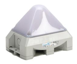
Pfannenberg PYRA series LED audible-visual signal beacon, 101 dB at 1m, (8) selectable tone(s), selectable permanent, blinking or flashing, red/yellow/green/blue, 166 x 114 x 134mm, 115-230 VAC, IP66, NEMA 4/4X.
