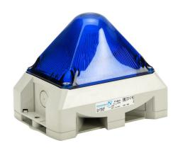
Pfannenberg PYRA series Xenon tube audible-visual signal beacon, 101 dB at 1m, (8) selectable tone(s), selectable flashing strobe, blue, 166 x 114 x 134mm, 10-57 VDC, IP66, NEMA 4/4X.
