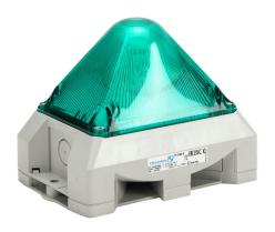
Pfannenberg PYRA series Xenon tube audible-visual signal beacon, 101 dB at 1m, (8) selectable tone(s), selectable flashing strobe, green, 166 x 114 x 134mm, 10-57 VDC, IP66, NEMA 4/4X.
