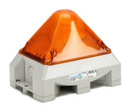
Pfannenberg PYRA series Xenon tube audible-visual signal beacon, 101 dB at 1m, (8) selectable tone(s), selectable flashing strobe, amber, 166 x 114 x 134mm, 10-57 VDC, IP66, NEMA 4/4X.
