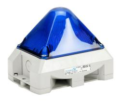
Pfannenberg PYRA series Xenon tube audible-visual signal beacon, 101 dB at 1m, (8) selectable tone(s), selectable flashing strobe, blue, 166 x 114 x 134mm, 115 VAC, IP66, NEMA 4/4X.
