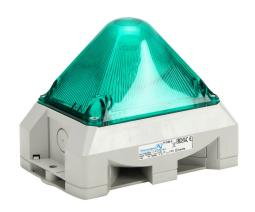
Pfannenberg PYRA series Xenon tube audible-visual signal beacon, 101 dB at 1m, (8) selectable tone(s), selectable flashing strobe, green, 166 x 114 x 134mm, 115 VAC, IP66, NEMA 4/4X.
