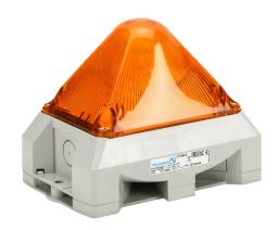
Pfannenberg PYRA series Xenon tube audible-visual signal beacon, 101 dB at 1m, (8) selectable tone(s), selectable flashing strobe, amber, 166 x 114 x 134mm, 115 VAC, IP66, NEMA 4/4X.
