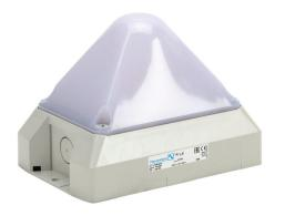
Pfannenberg PYRA series LED industrial signal beacon, 166 x 114 x 124mm, red/yellow/green/blue, selectable permanent, blinking or flashing, IP66, NEMA 4/4X, surface mount, 12-48 VDC.
