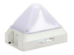
Pfannenberg PYRA series LED industrial signal beacon, 166 x 114 x 124mm, red/yellow/green/blue, selectable permanent, blinking or flashing, IP66, NEMA 4/4X, surface mount, 115-230 VAC.
