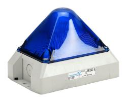
Pfannenberg PYRA series Xenon tube industrial signal beacon, 166 x 114 x 134mm, blue, selectable flashing strobe, IP66, NEMA 4/4X, surface mount, 10-57 VDC.
