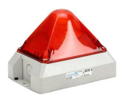
Pfannenberg PYRA series Xenon tube industrial signal beacon, 166 x 114 x 134mm, red, selectable flashing strobe, IP66, NEMA 4/4X, surface mount, 10-57 VDC.
