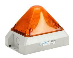
Pfannenberg PYRA series Xenon tube industrial signal beacon, 166 x 114 x 134mm, amber, selectable flashing strobe, IP66, NEMA 4/4X, surface mount, 10-57 VDC.
