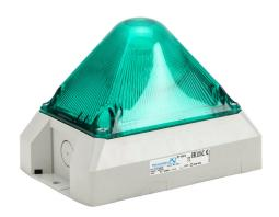
Pfannenberg PYRA series Xenon tube industrial signal beacon, 166 x 114 x 134mm, green, selectable flashing strobe, IP66, NEMA 4/4X, surface mount, 115 VAC.
