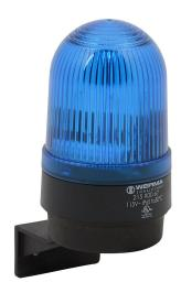
WERMA Xenon tube industrial tall signal beacon, 58mm, blue, flashing strobe (0.75 Hz flash frequency), IP65, bracket mount, 115 VAC.
