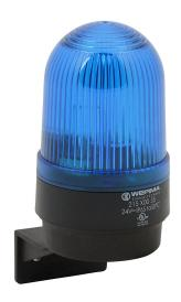
WERMA Xenon tube industrial tall signal beacon, 58mm, blue, flashing strobe (0.75 Hz flash frequency), IP65, bracket mount, 24 VDC.
