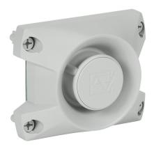
Pfannenberg PYRA series audible signal horn, 105 dB at 1m, 150–2900 kHz tone frequency, (80) selectable tone(s), 115 VAC, polycarbonate housing, gray, IP66, NEMA 4/4X. For use with Pfannenberg PYRA series pre-assembled bases.
