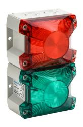
Pfannenberg PYRA series LED traffic light, (2) tiers, red/green, selectable permanent, blinking or flashing light function, 115-230 VAC, colored lens, 172.4mm body length, light gray, direct mount, IP66, NEMA 4/4X.
