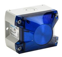
Pfannenberg PYRA series Xenon tube industrial signal beacon, 109 x 86 x 80mm, blue, flashing strobe (1 Hz flash frequency), IP66, NEMA 4/4X, surface mount, 24 VDC.
