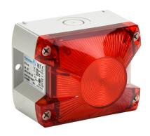
Pfannenberg PYRA series Xenon tube industrial signal beacon, 109 x 86 x 80mm, red, flashing strobe (1 Hz flash frequency), IP66, NEMA 4/4X, surface mount, 24 VDC.
