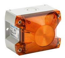
Pfannenberg PYRA series Xenon tube industrial signal beacon, 109 x 86 x 80mm, amber, flashing strobe (1 Hz flash frequency), IP66, NEMA 4/4X, surface mount, 24 VDC.
