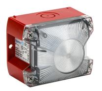
Pfannenberg PYRA series Xenon tube industrial signal beacon, 109 x 86 x 80mm, clear/white, flashing strobe (1 Hz flash frequency), IP66, NEMA 4/4X, surface mount, 24 VDC.
