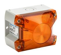
Pfannenberg PYRA series Xenon tube industrial signal beacon, 109 x 86 x 80mm, amber, flashing strobe (1 Hz flash frequency), IP66, NEMA 4/4X, surface mount, 115 VAC.
