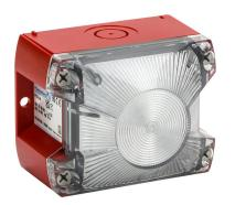
Pfannenberg PYRA series Xenon tube industrial signal beacon, 109 x 86 x 80mm, clear/white, flashing strobe (1 Hz flash frequency), IP66, NEMA 4/4X, surface mount, 115 VAC.
