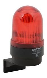
WERMA Xenon tube industrial tall signal beacon, 58mm, red, flashing strobe (0.75 Hz flash frequency), IP65, bracket mount, 24 VDC.
